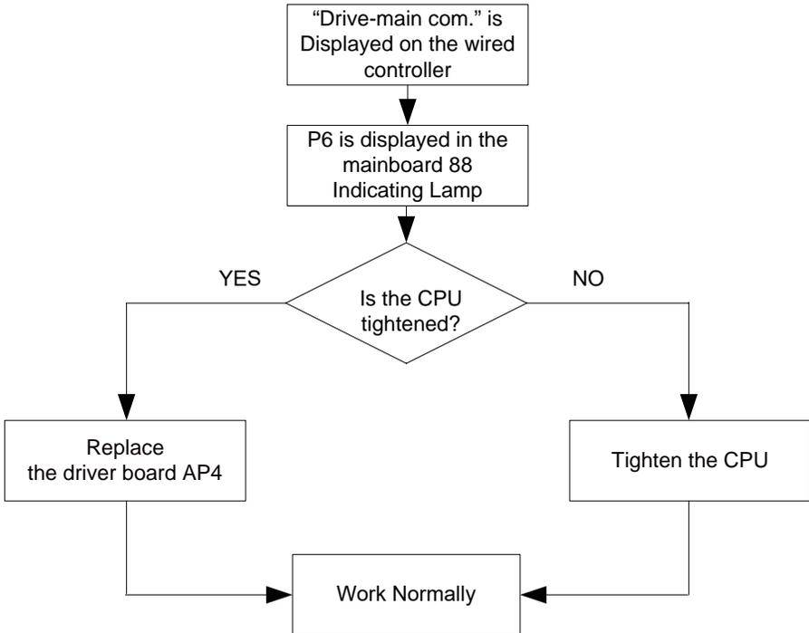
◆ Compressor Startup Failure(code:"LC")
