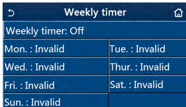
2. At the “Weekly timer” setting page, as shown in the figure below, the weekly timer can be set to “On” or “Off”.
