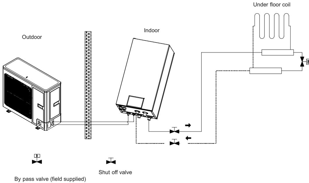
Note: the bypass valve must be installed to secure enough water flow rate, and should be installed at the collector.
