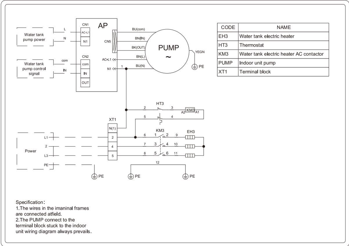
4.10 Wiring of the Terminal Board
