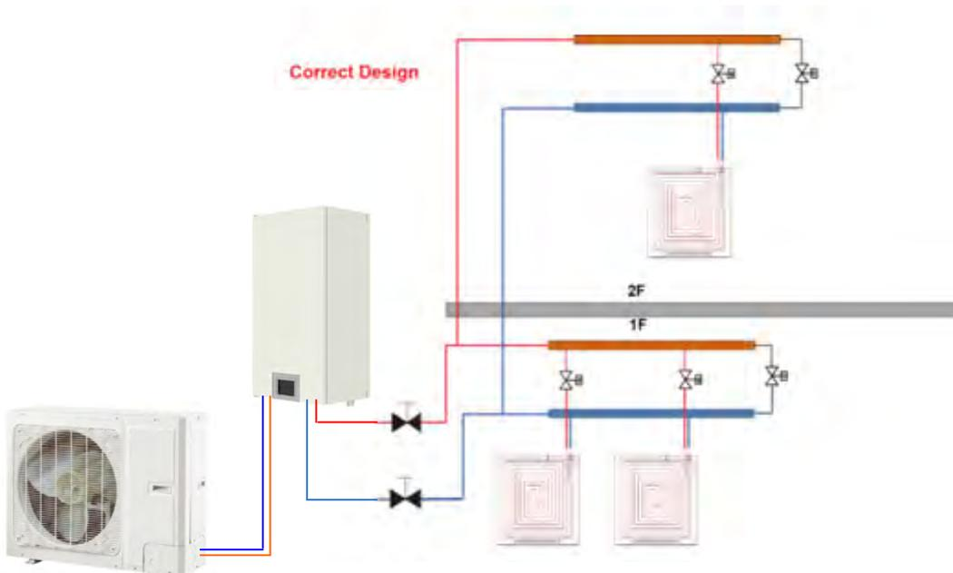
(5) Distance between the unit and the water manifold should be within 15m. If the distance exceeds 20m, then it is required to calculate the hydraulic power.
