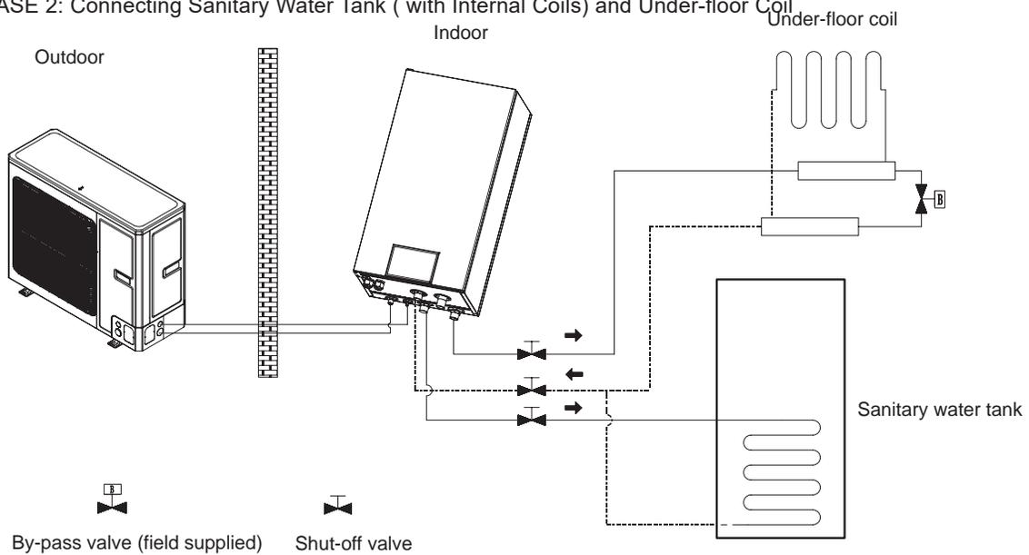
Note: sanitary water tank should be equipped with internal electric heater to secure enough heat energy in the very cold days.
