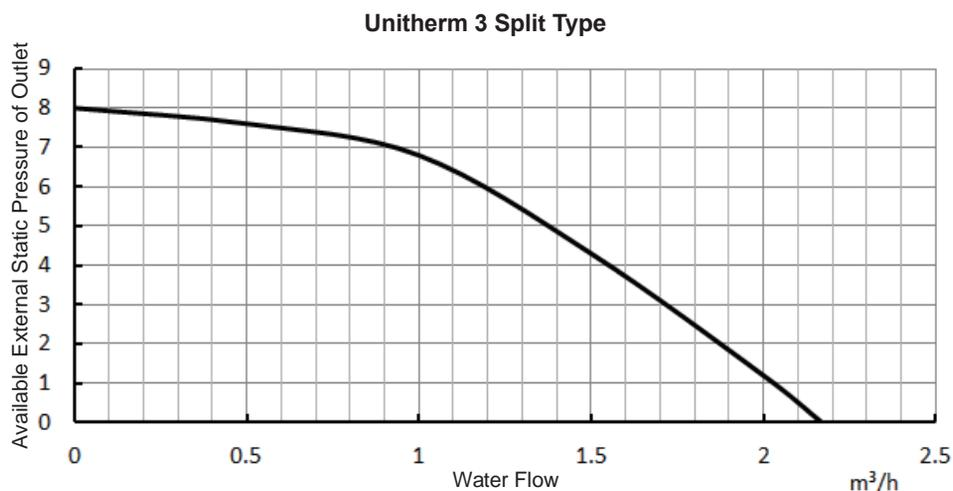
Note: see the curve above for the maximum external static pressure. The water pump is of variable frequency. And during operation, the water pump will adjust its output based on the actual load.
