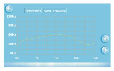
Temperature curve automatically updates every one hour, and the curve record can be stored for 60 days; Start from the latest curve saved time, if power is off and curve data collecting time is less than one hour, the data in this period will not be saved;
