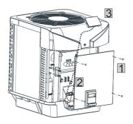
Notes: Touch display installation for magnetic adsorption, can be directly removed
