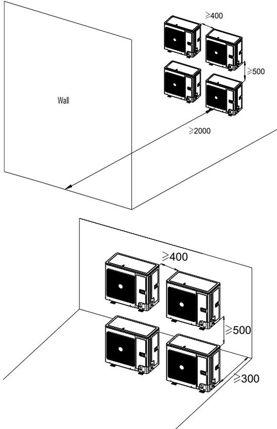
(2) Diagram of installation location and space for indoor unit (Notice: for the best performance of indoor unit, make sure its installation space conforms to the following installation dimensions).
