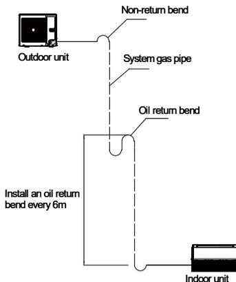
Dimensions for the making of oil return bend are as follows:
