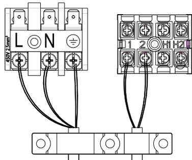
Remove the big handle/front panel of the outdoor unit and insert one end of the communication cord and the power cord to the terminal board.
