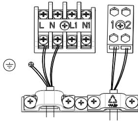
b) Wire routing of unified power supply:
