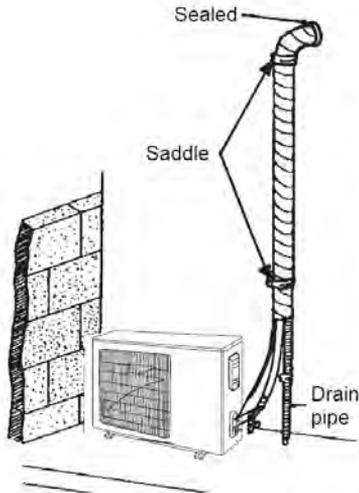
(2) If the outdoor unit is above the indoor unit, arrange the pipeline according to the following diagram.
